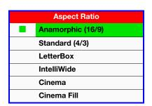
To change the aspect ratio (size and shape) of the projected image, select Aspect Ratio from the Main Menu and press **ENTER**. Select the appropriate aspect ratio for the type of program material being viewed; refer to Table 4-1.
